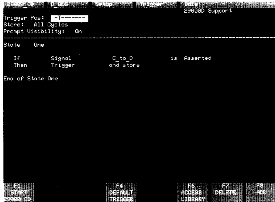
Figure 4-4. Trigger program default setup for the D_Bus module. This trigger program is also for the 29000_9696 setup.
